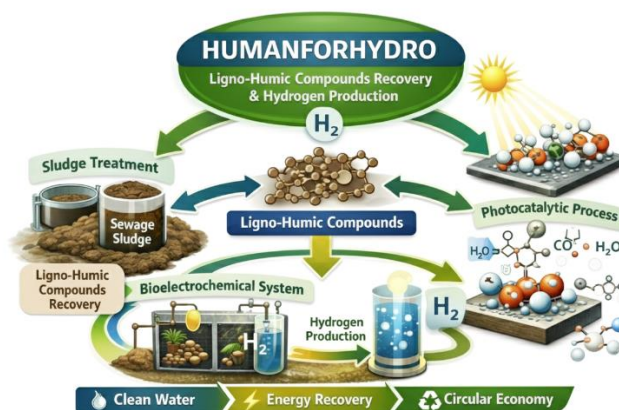
Figure 1. Schematic of the HUMANFORHYDRO project showing LHL recovery from sewage sludge and their use in bioelectrochemical and photocatalytic systems for hydrogen production and pollutant removal.
