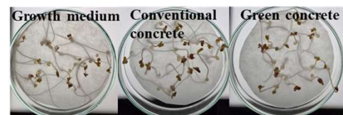
Mustard seed roots after germination test in 100 g L -1 concrete leachates.
