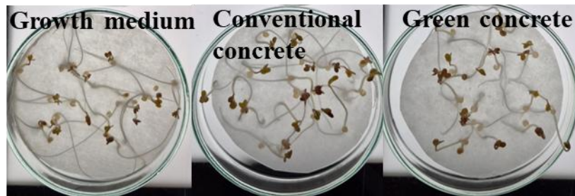
Figure 2. Mustard seed roots after germination test in 100 g L -1 concrete leachates.
