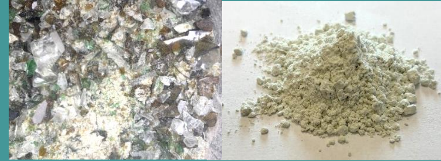
Figure 1. Crushed glass in two crushing phases
