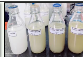
Dairy Wastewater Cultures during the Batch Microbial Treatment (Mixed Culture of R1 & R3) Integrated with Psidium guajava Leaves Extract
